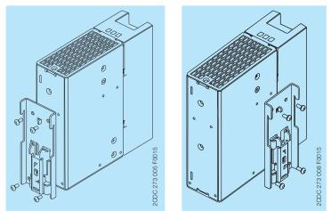
To mount the unit in position 7 remove the DIN rail adapter that is fastened with 4 screws and attach it on the side of the power supply.
